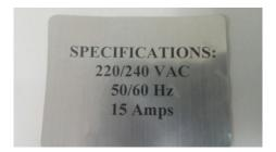
Located under the machine at the foot end, where the power cord is inserted.
