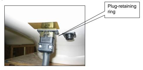
Figure 4.7.1 Connection of Power Cord
